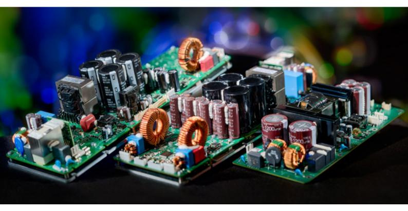
Class D amps are often mistakenly referred to as digital amplifiers because this approach to decimated waveform reproduction bears a great deal of similarity to the way sampled digital audio is stored and reproduced. Essentially it uses a very fast series of rectangular pulses to represent the amplitude and timing characteristics of the waveform instead of simply amplifying the original waveform signal shape intact.
